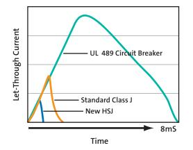
Compared to fuses, circuit breakers do very little to limit the let-through energy (I2t) of a fault condition, which can lead to extensive damage.
