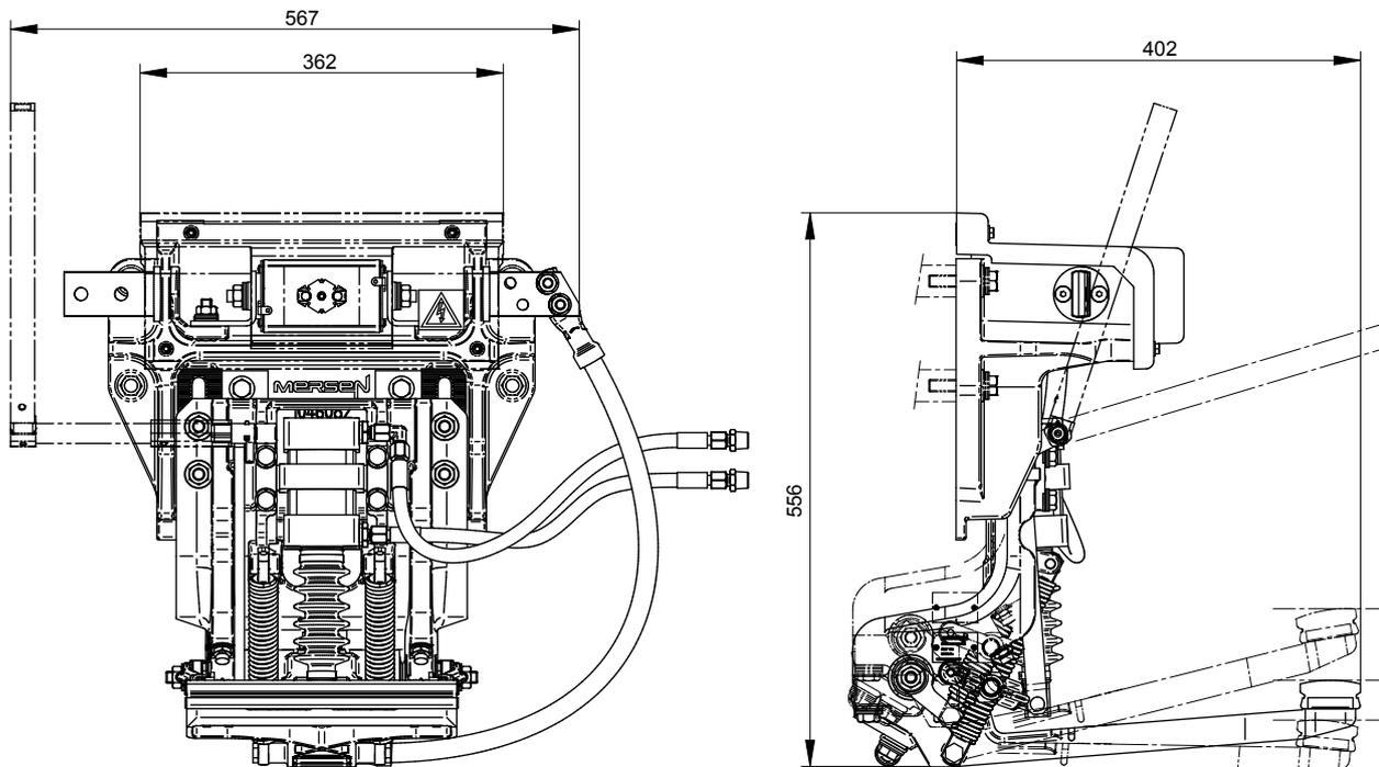
Compact and pneumatic retraction with integrated fuse box - contact from the bottom
