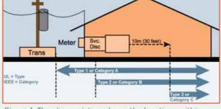
Figure 1: The above picture shows the locations within the electrical distribution and the associated Type device adopted by IEEE categories A, B, & C
