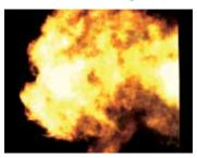
A 22.8kA fault current is delivered to a circuit protected by a circuit breaker with a clearing time of 6 cycles. The resulting incident energy measured at 18" from the conductors was 8.14 cal/ cm<sup>2</sup>, making Category 3 the minimum PPE required.
